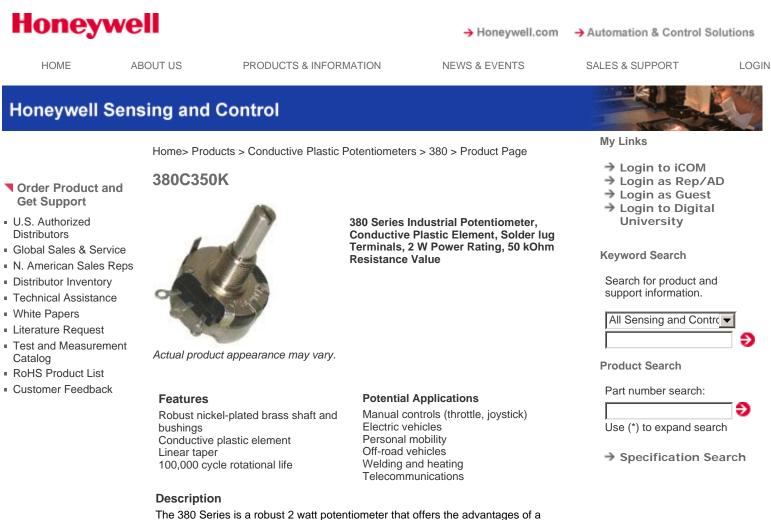
conductive plastic element and a 100,000 cycle rotational life. Special tapers and element designs available on a special order.
